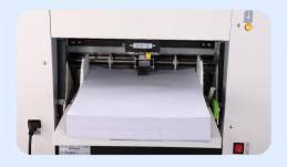
Precise paper feeding pressure adjustment realize excellent printing of various paper types, from 40g-157g/m2. Three shifts pressure adjustment from thin paper to thick paper enhances reliability.
